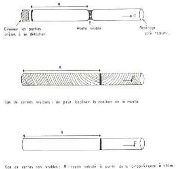
Figure 4. Location of the pith and Core length before cutting
