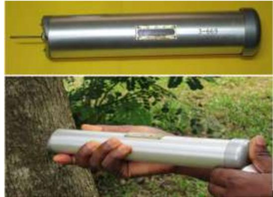
Figure 3: The wood tester pilodyn of a capacity of 6 joules used for the experimentation
